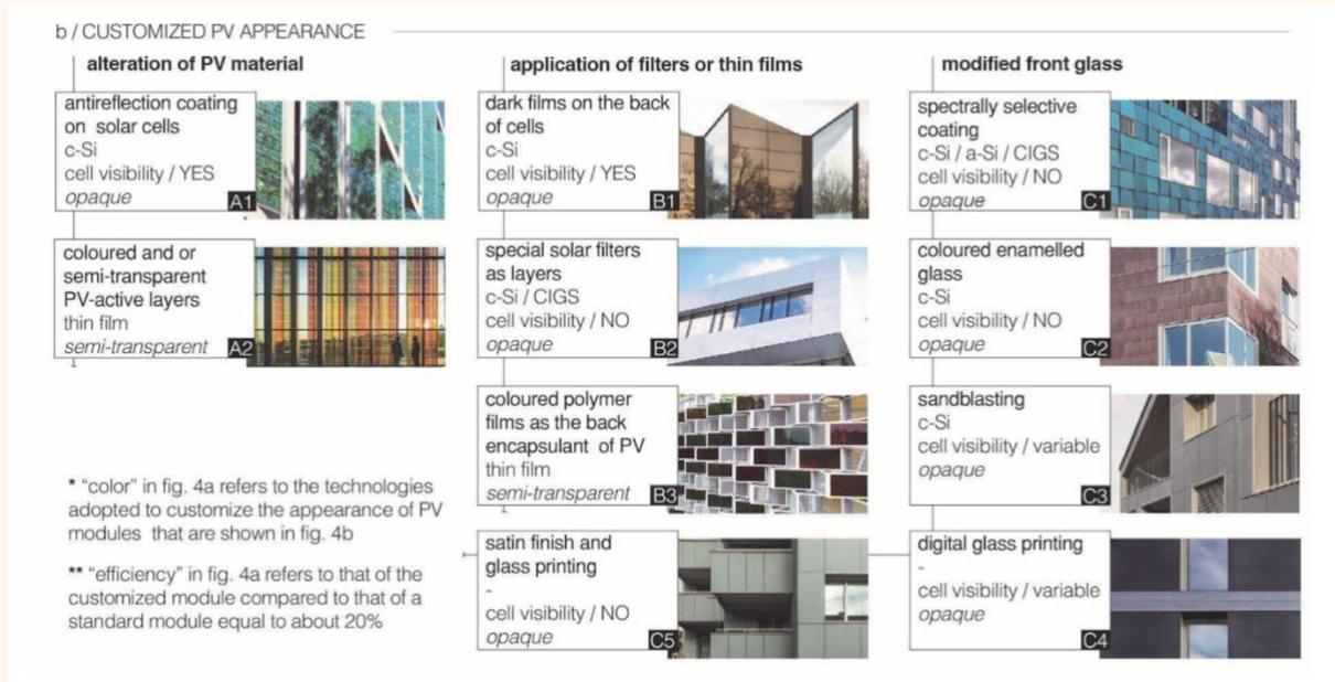
**Figure 8.** PV products overview. The graphic illustrates the current colouring technologies for PV components and the range of different formal interpretations. Original graphics by Guido Callegari, Politecnico di Torino.
