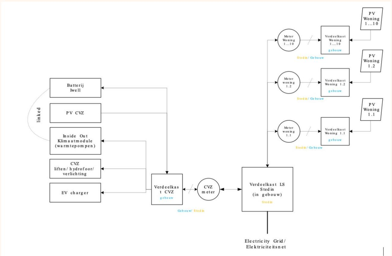
**Figure 52.** Setup of the energy system and EMS control in one of the buildings in Utrecht, where this solution has been implemented (Henriette-dreef building).
