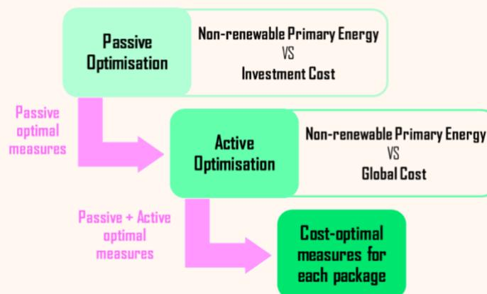
*Figure 25. The conceptual scheme adopted for integrated energy design.*
