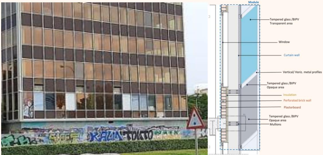
**Figure 53.** Picture of the GESA building façade and the proposed modular prefabricated façade with BIPV, as a result of solutions analyzed under an integrated energy design approach
