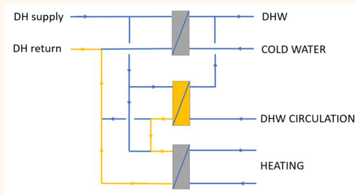
Figure 10. Operating diagram of the aftercooling system
