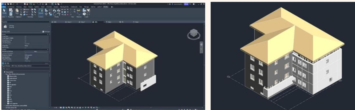
*Figure 55. Demo case in Trento, Italy: the existing building (top) and the consistent BIM used for designing the refurbishment intervention in Autodesk Revit (bottom)*
