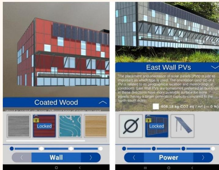
*Figure 34. Screenshots of the AR tool showing information about different façade elements/materials.*
