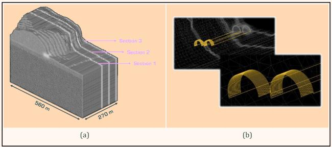
*Figure 56.* Illustration of (a) the numerical model and (b) close-up view of the heat exchanger system configuration in Section 2 located at an average distance of 65 m from the tunnel mouth.
