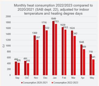
Figure 48. Monthly heat consumption in two time periods.
