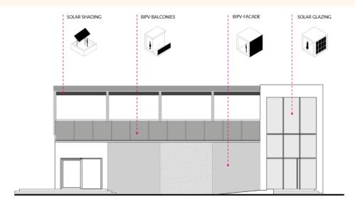
*Figure 6.* Photovoltaic integration forms identified on the envelope of the Demo Project Trento, South facade. Original graphics by Guido Callegari, Politecnico di Torino.
