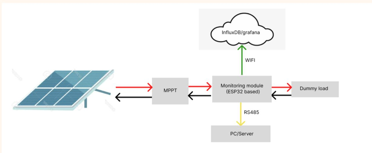
Figure 23. BIPV Monitoring concept
