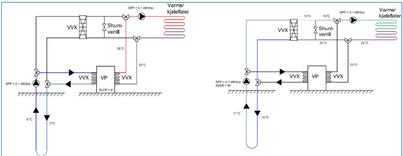
**Figure 19.** Schematic of the LowEx system, in winter operation (left) and summer operation (right).
