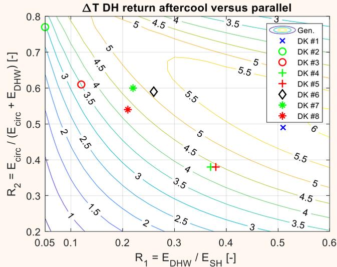
**Figure 11.** Calculated yearly building level district heating return temperature reduction potential.
