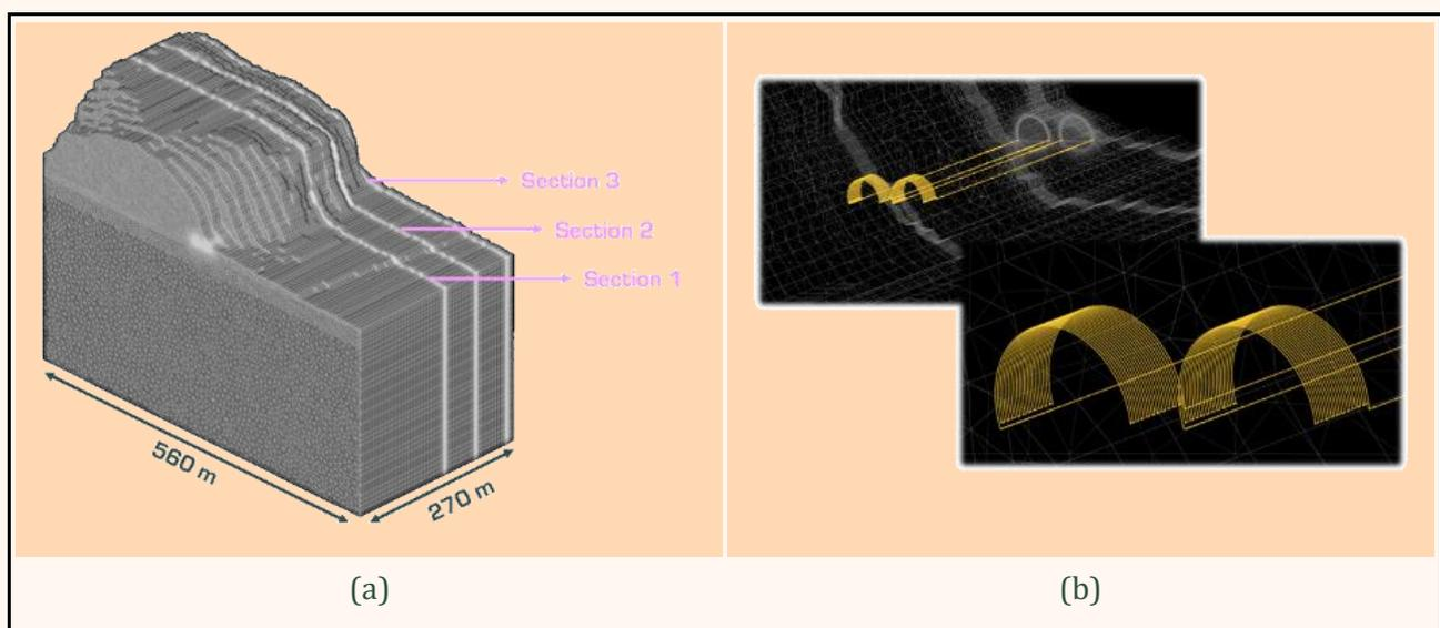
**Figure 56.** Illustration of (a) the numerical model and (b) close-up view of the heat exchanger system configuration in Section 2 located at an average distance of 65 m from the tunnel mouth.
