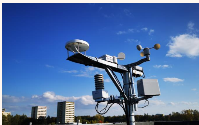
Fig. 13 The weather station setup includes a sky-imager and a reference solar irradiance sensor.
