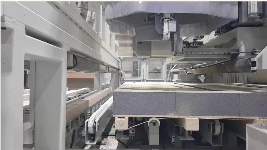
Figure 53. The CNC Cutting machine which creates the Rc Panels façade element.
