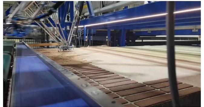
Figure 56. Left: Overview of the stone slip laying robot at Rc Panels, featuring a prefabricated façade to receive stone slips. Right: Close-up of the stone slip laying robot at Rc Panels.
