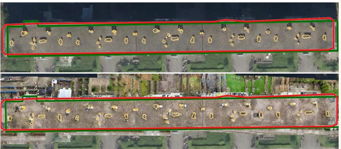
Figure 12. Source aerial imagery of Alexander de Grotelaan 1-129 with Rooftop Recognition predictions overlay of roof ducts versus stitched georeferenced picture by DJI mini pro 4 drone. Green is BAG building footprint, Red is rooftop segmentation, Yellow is object segmentation.
