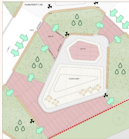
Figure 15. Scheme of storm water management in one of the project's islands. Original image by ØSTENGEN & BERGO AS, edited by Nicola Lolli (SINTEF).
