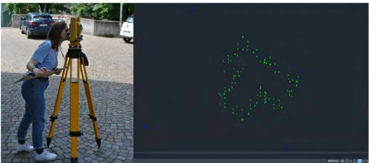
Figure 2 – On the left, the total station in use. On the right, blue points represent the 4 stations, green ones represent points acquired during the topographic survey.
