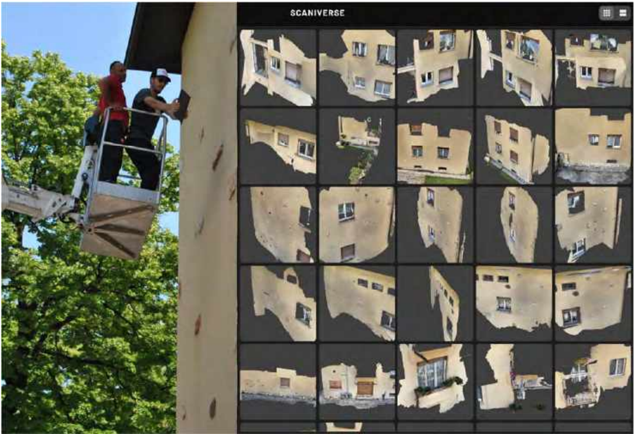
Figure 4 – On the left, the iPad in use. On the right, some scans acquired with Scaniverse application.
