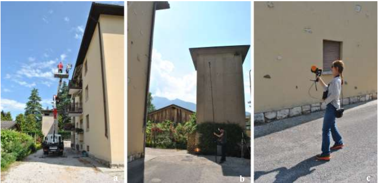
Figure 44. Scanning with LiDAR technology from the aerial platform (a); acquiring pictures with the 3DEye system (b); scanning with SLAM technology from ground level (c). Source: UNITN.
