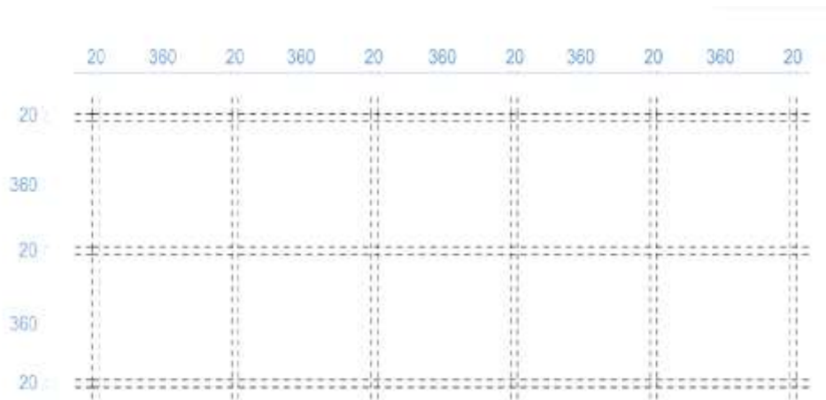
Figure 21. Module and construction grid for the redefined New Building. Source: UNITN.
