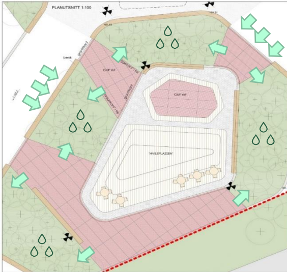
Figure 27. Scheme of storm water management in one of the project's "islands". Original image by ØSTENGEN & BERGO AS, edited by Nicola Lolli (SINTEF).
