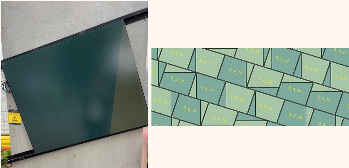
Figure 35. Left: image of one of the bi-coloured PV panels tested on the building site (photo by Inger Andresen, NTNU). Right: technical section of the school façade. Right: scheme of different installations of the two bi-colour PV panels. Original image by KONTUR and SPINN Arkitekter, edited by Nicola Lolli (SINTEF).
