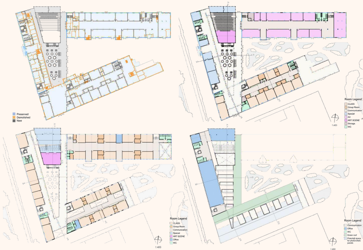
Figure 62. Blue: preserved / Orange: demolished / Gray: new // floor plan of the ground floor
