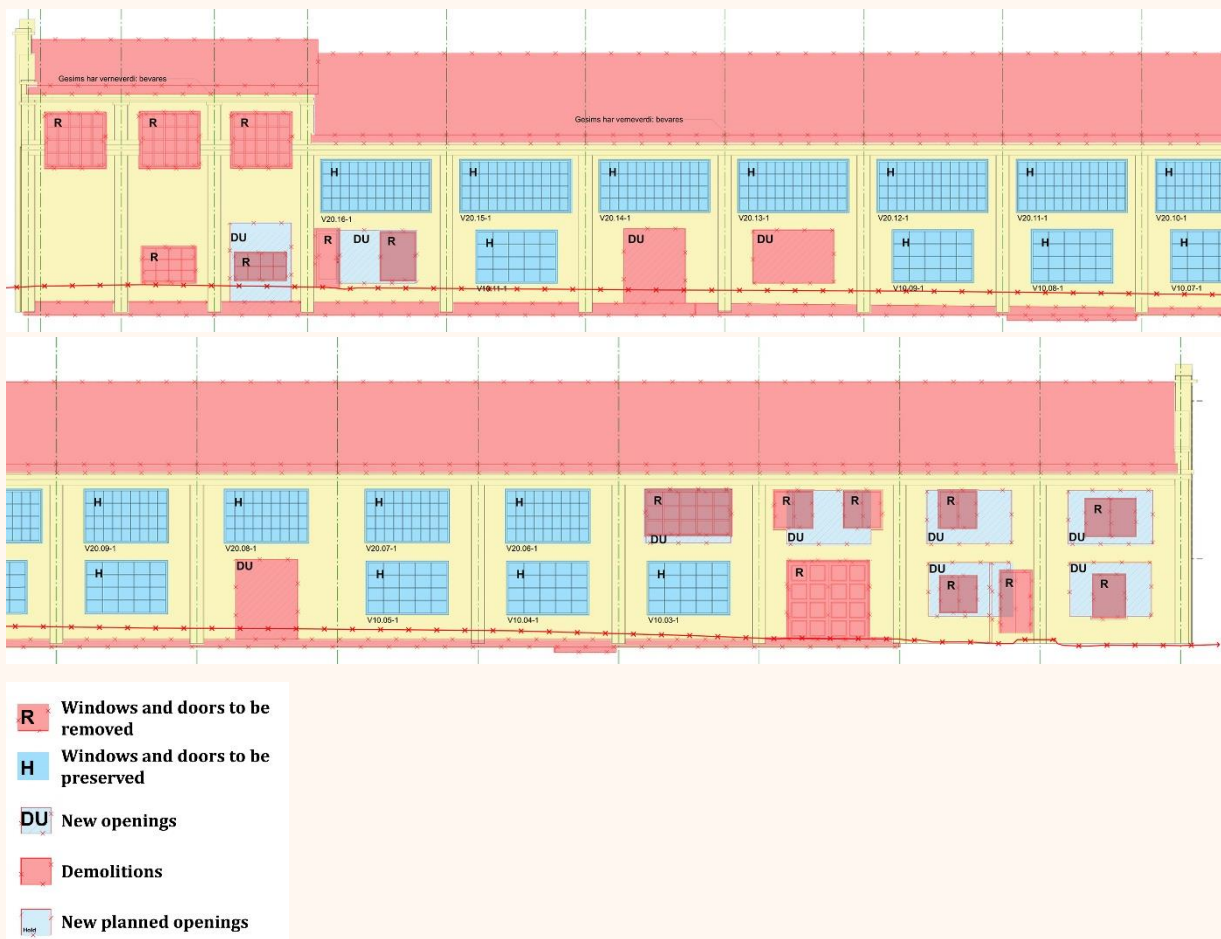
Figure 24. Demolition plan of the north façade of Heidenreich building. Original image by KONTUR and SPINN Arkitekter, edited by Nicola Lolli (SINTEF).
