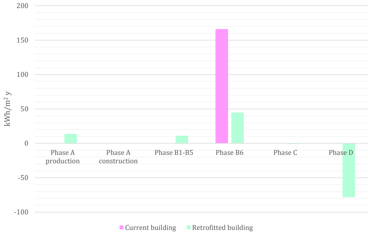
Figure 48. Cumulative energy demand of the building before and after the retrofit. Only building-related energy demand is included.
