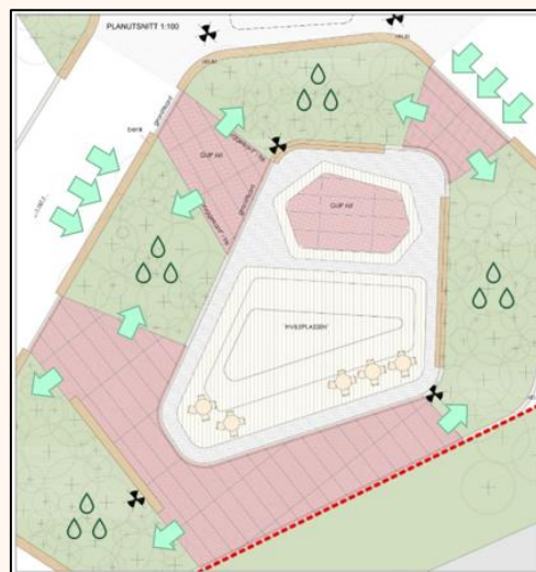
Figure 10. Scheme of storm water management in one of the project's "islands". Original image by ØSTENG & BERGO AS, edited by Nicola Lolli (SINTEF).
