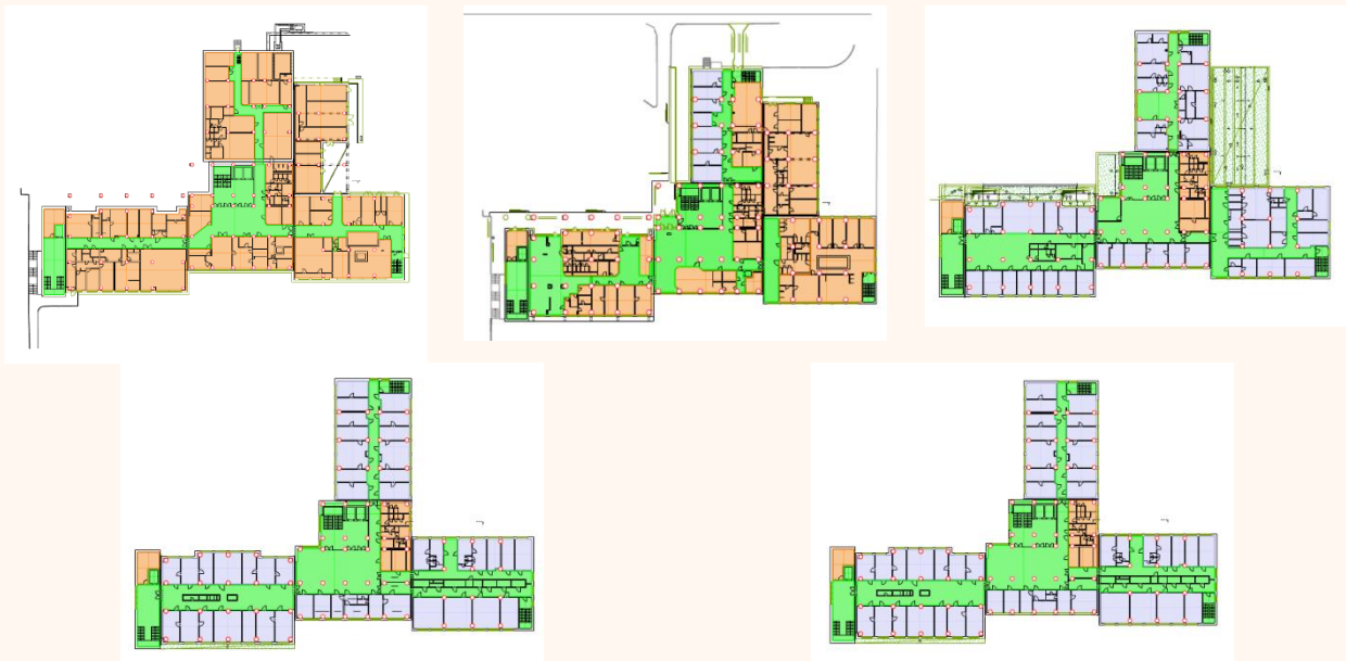
Figure 33. Ongoing zoning of the demo building for energy simulations
