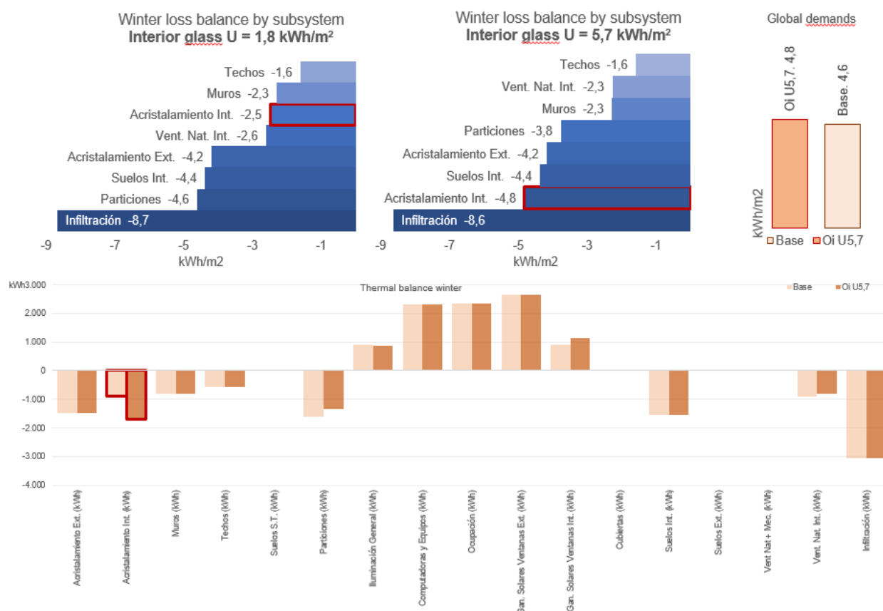
Figure 54. Comparison of the internal loss balance depending on the performance of the glass. Extracted from the project documentation (partly in Spanish language 6 ).
