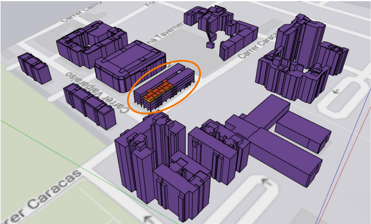
Figure 20. The building model with a shading effect from nearby buildings (Archetype 1).
