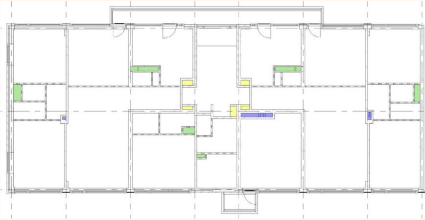
Figure 9. Central vertical ducts (as part of the HVAC system)
